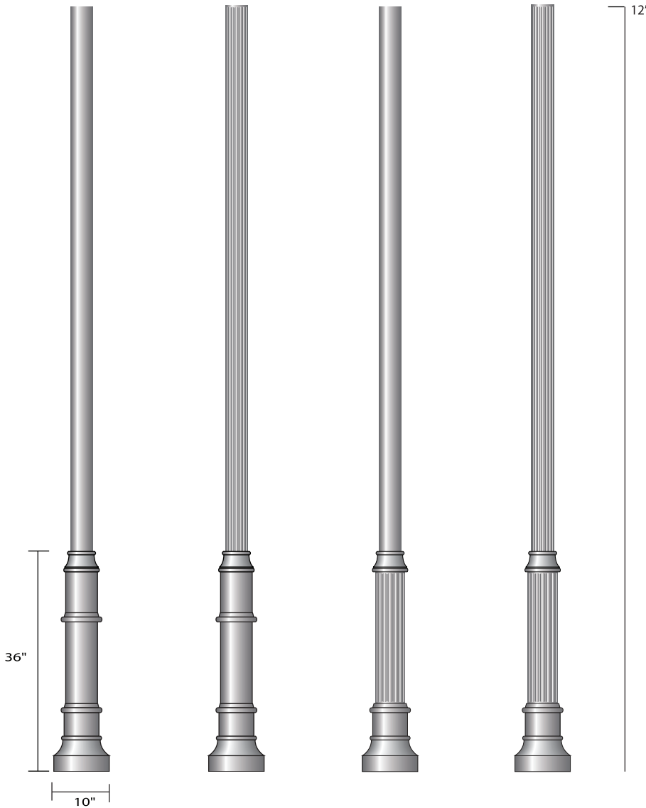
3-4" O.D. SMOOTH INTO SMOOTH ALUMINUM 12" MAXIMUM HEIGHT
