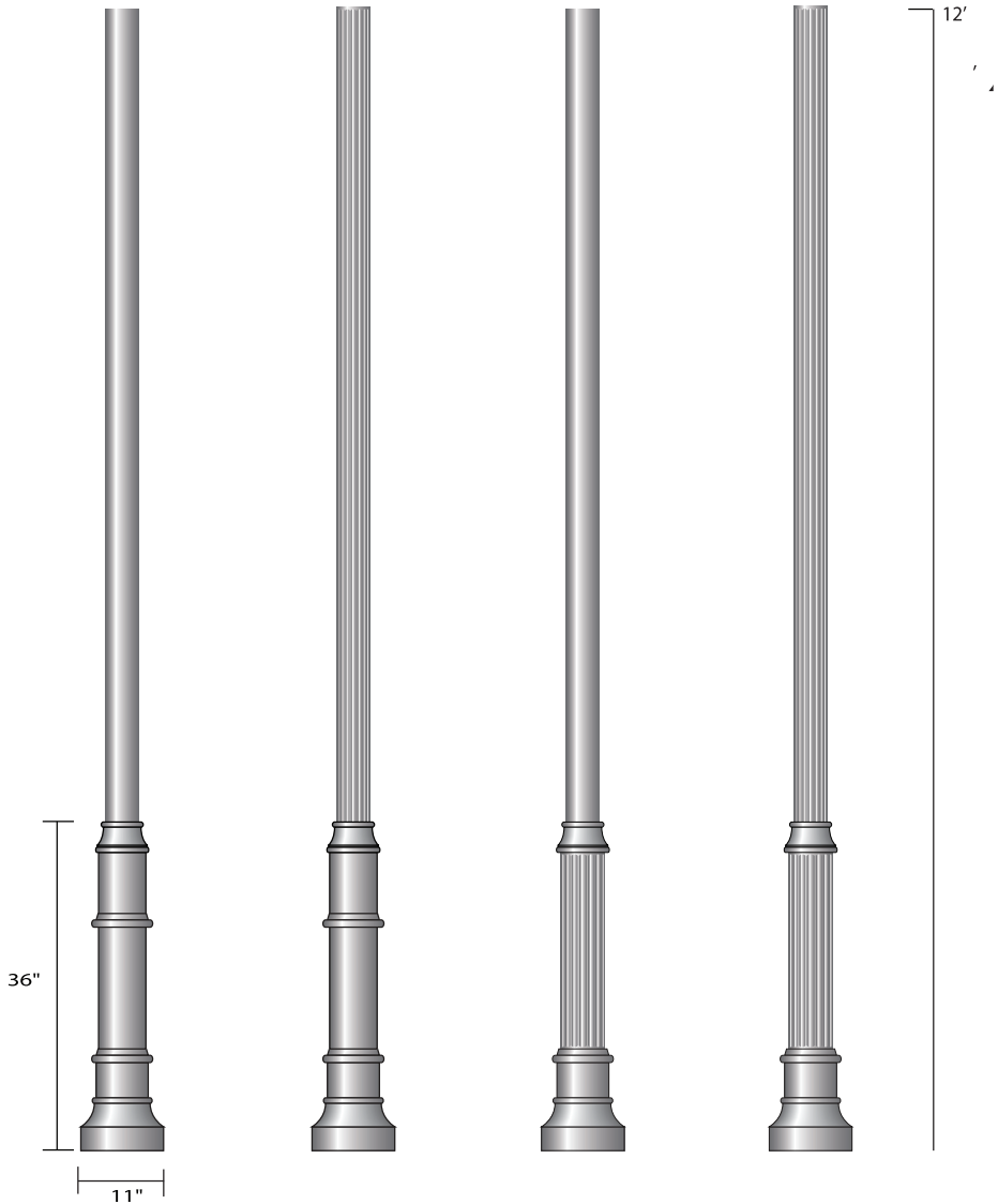
3'-5" O.D. SMOOTH INTO SMOOTH ALUMINUM 12" MAXIMUM HEIGHT
