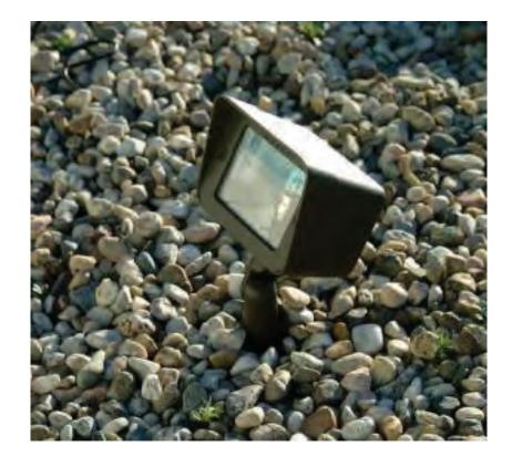
Fully adjustable locking knuckle so you can always get the angle you need and keep it there. Clear acrylic lens is fully gasketed, to provide a tight fit against moisture. Includes a diamond embossed specular aluminum reflector to provide the perfect amount of light for your project.
