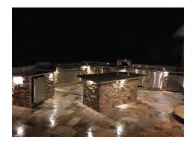
The LED Hardscape Light Series consists of four; very low profile strip lights, available in various lengths and colors. Their durable and flexible designs enable mounting under capstones, railings, benches, and other hardscape applications. They can also be used for rooftop landscape mounting as well. These lights deliver exceptionally wide, diffused illumination without hot spots. They provide a diverse range of lighting solutions and are essential additions to the lighting designer's toolset.
